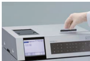
Calibration by magnetic card
